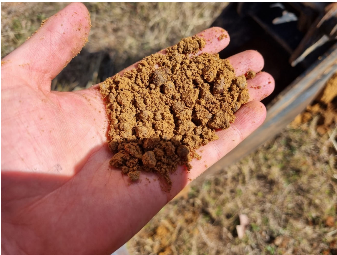
Photo 6 – Silty, Gravelly Clay from TP1
